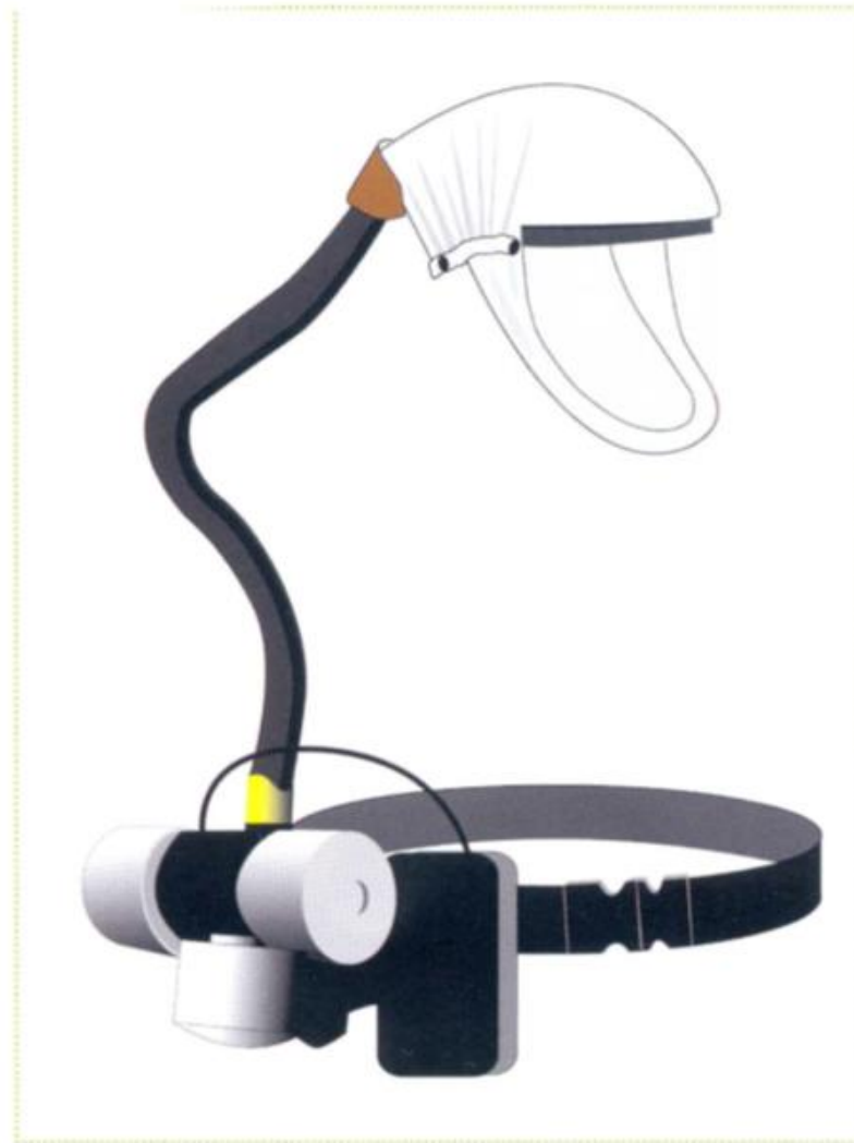
Personal protection measures: schematic drawing of a power air purifying respirator (PAPR)
